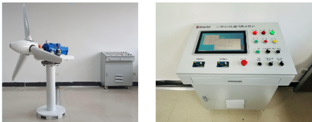
Figure 4 Direct Drive Wind Turbine and Control Panel of the New Energy Center
